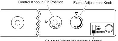
Selector Switch in Remote Position (Optional Remote Control)
